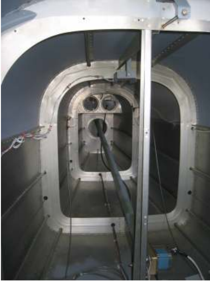
Fasten wires for magnetometer and drill holes for it.
