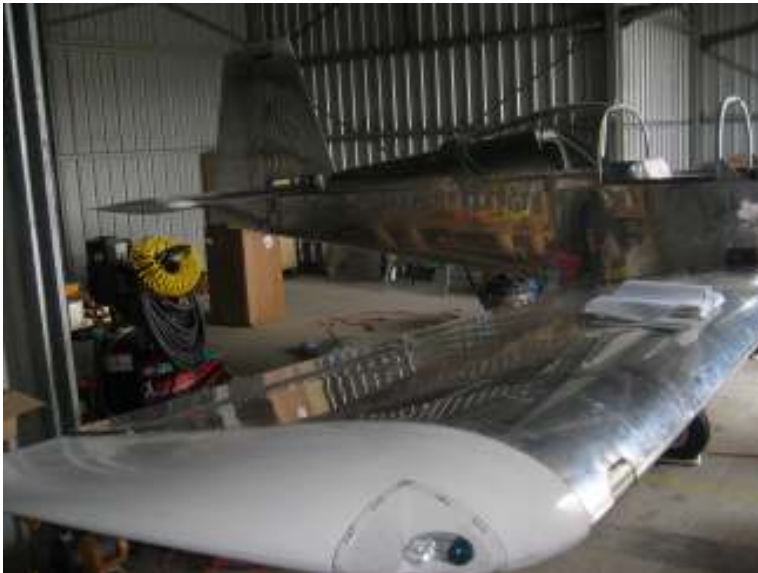
Install wing tips (left wing tip missing one nutplate) Total time: 4 hours (1324 hrs)
