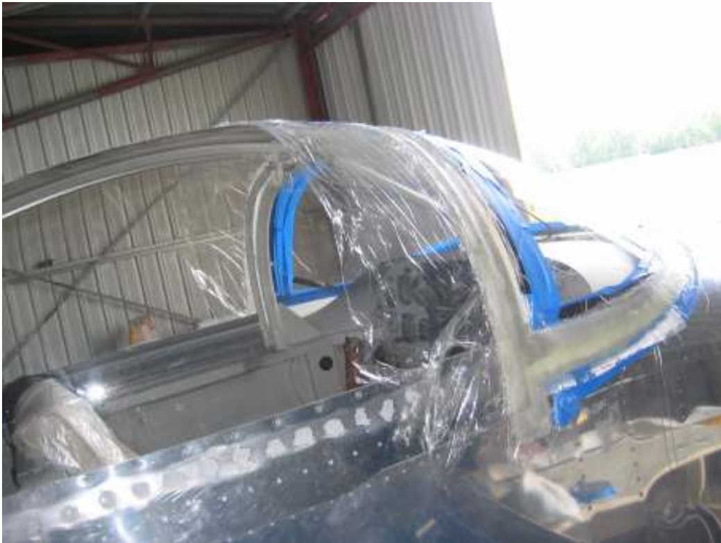
Laying fiber glass at the top Sand some fiber glass at the base of the windshield Add Adel clamps for mag cables
