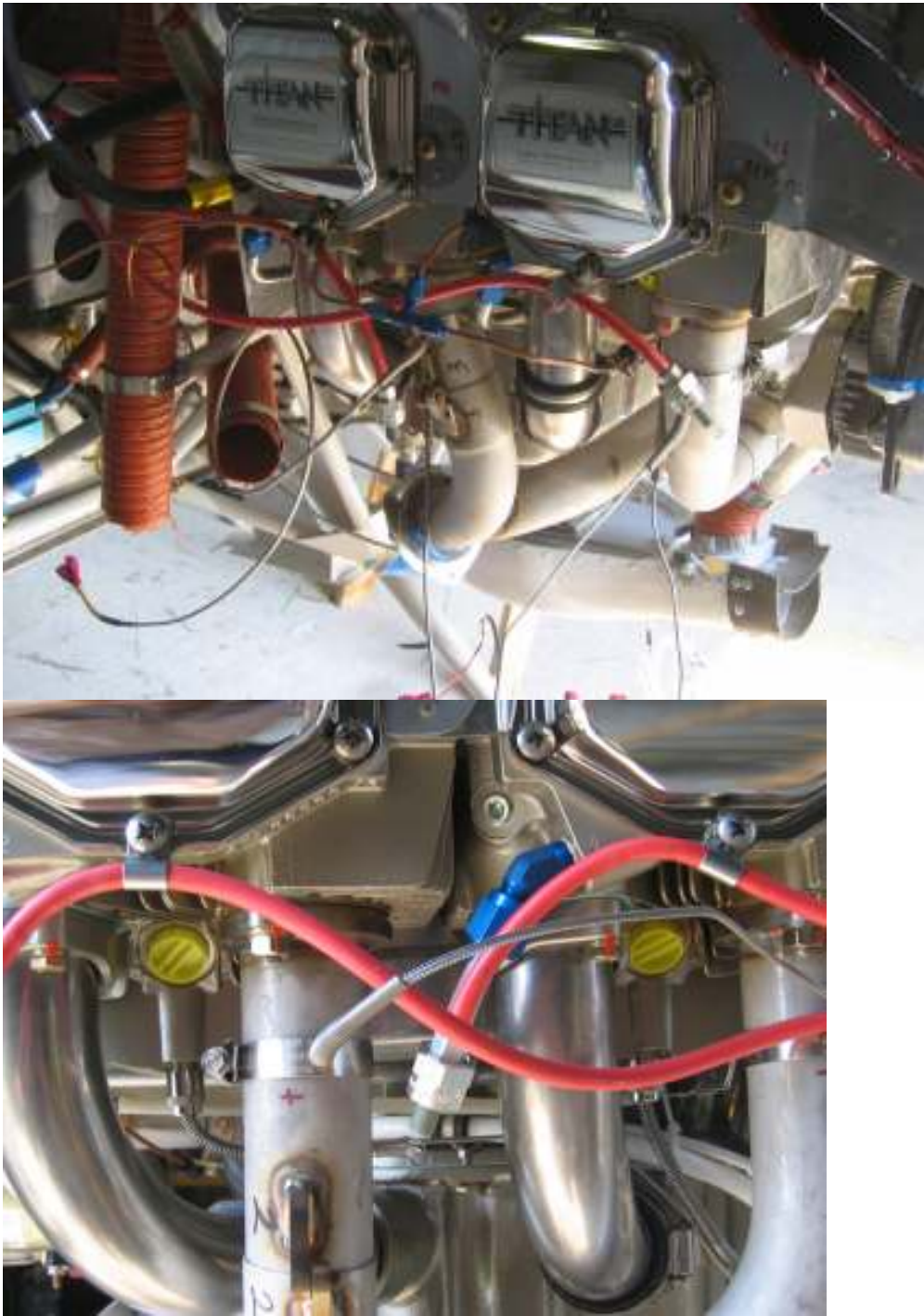
Install oil temp, CHT, EGT probes
