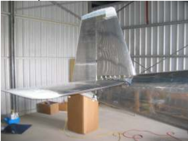
Install trim tab and reinstall left elevator Total time: 3 hours (1327 hrs)
