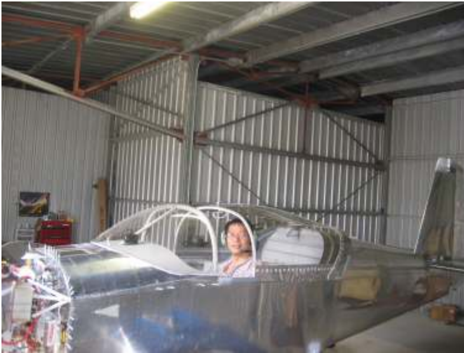
Install windshield and bar on roll bar Install compass and windshield antenna
