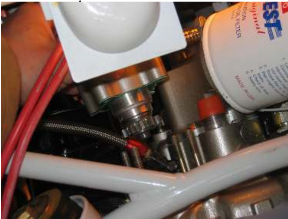
Connect oil pressure line (first take out vacuum port to install the restrictor)
