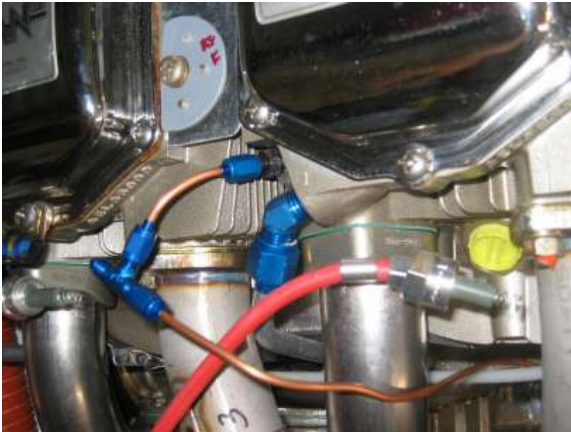
Partially install prime line (waiting for fuel pressure line location)
