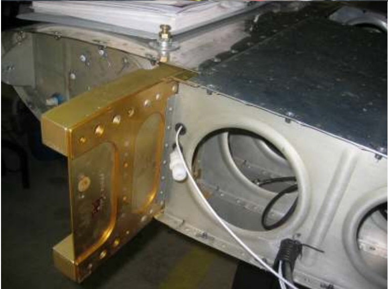
Pitot line connection (both end at wing done)
