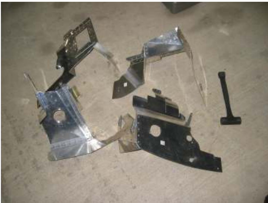
Make and rivet bottom reinforcement tabs
