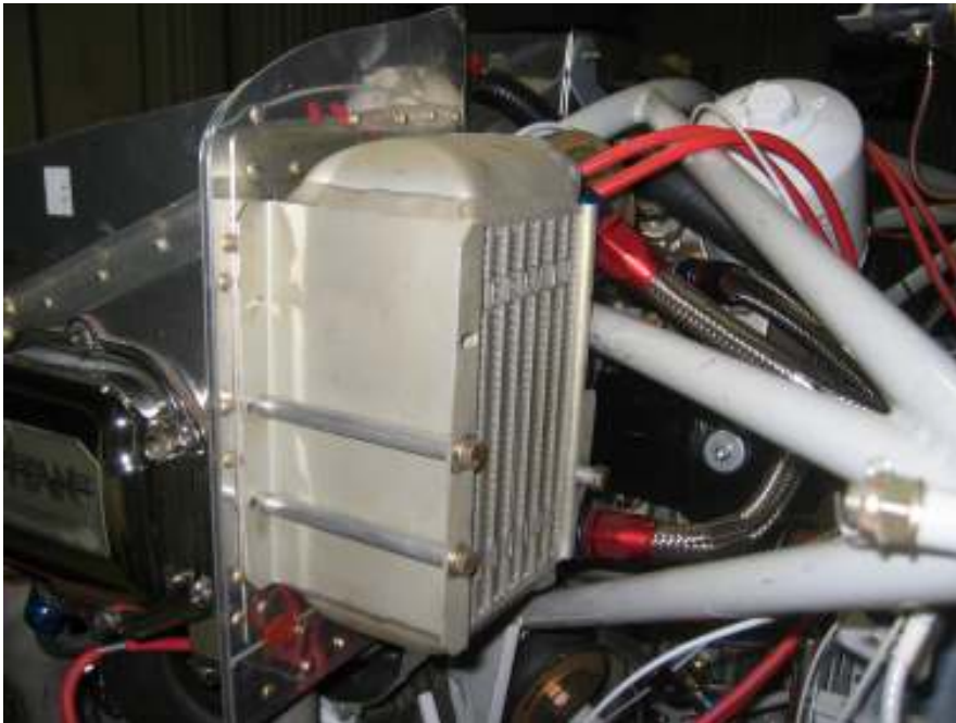
Cut oil cooler spacers and mount oil cooler Total time: 7 hours (948 hrs)
