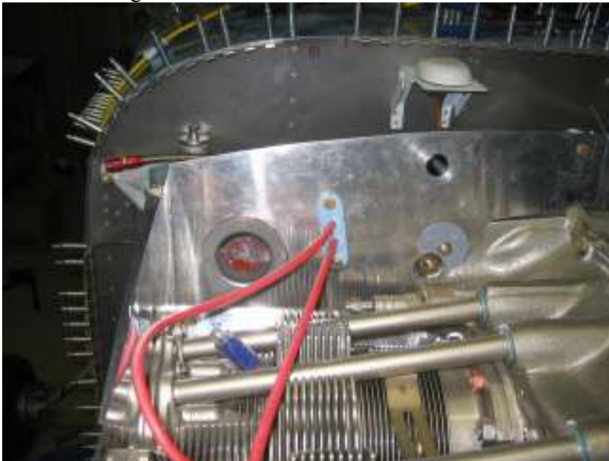
Drill Mag lead hole
