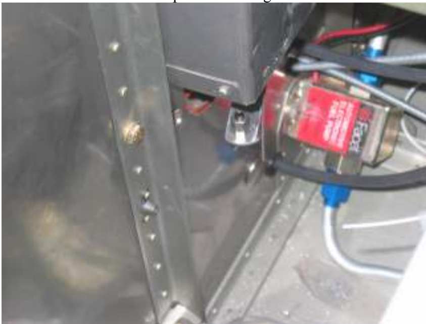
Install nuts for cabin heat door
