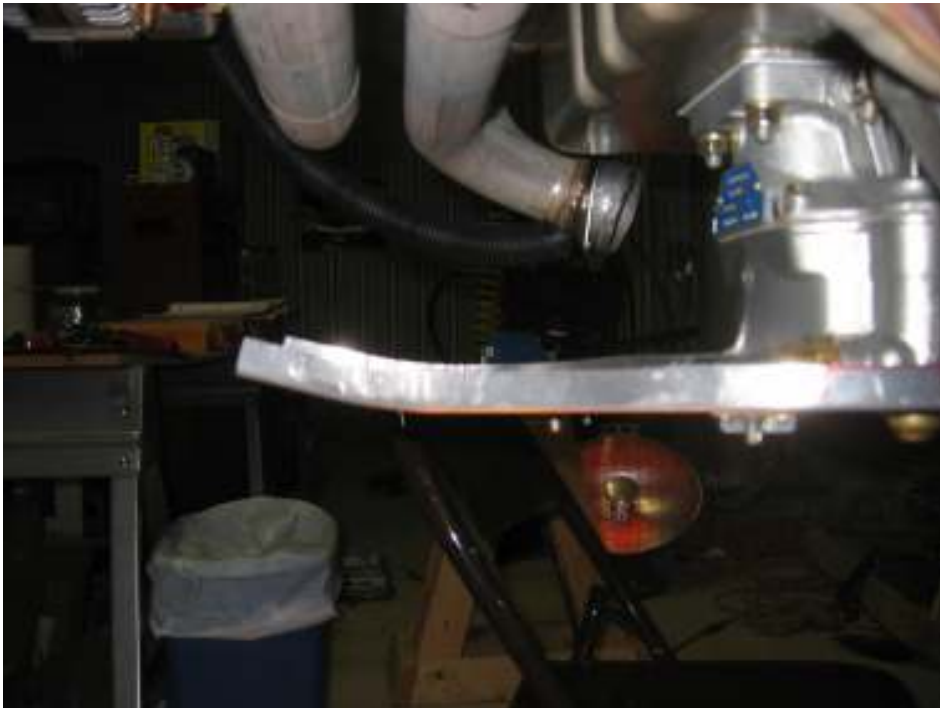
Shrink top plate to curve up and align with inlet Trim air box
