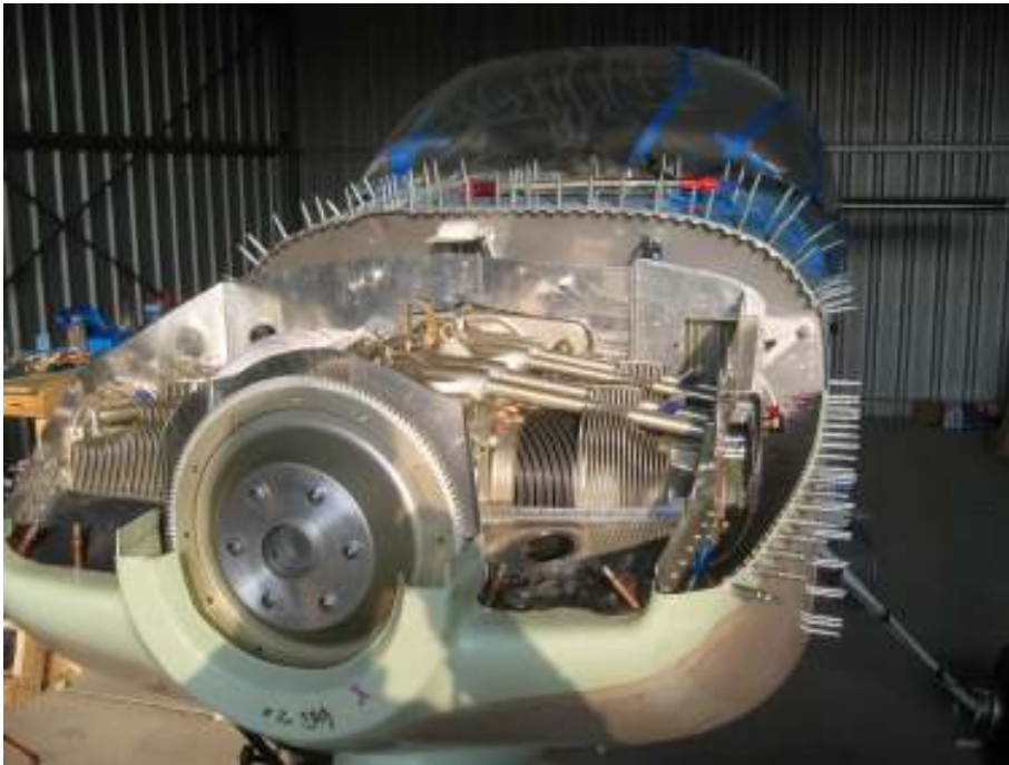
Rivet baffle parts together, trim again Trim inlet and add airseal at inlet
