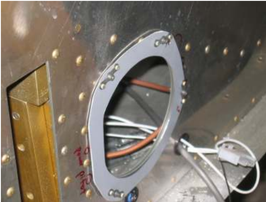
Install platenuts on aileron push rod boot retainers
