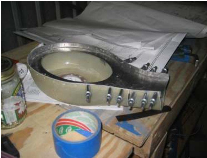
Drill rivet holes on air box and top plate
