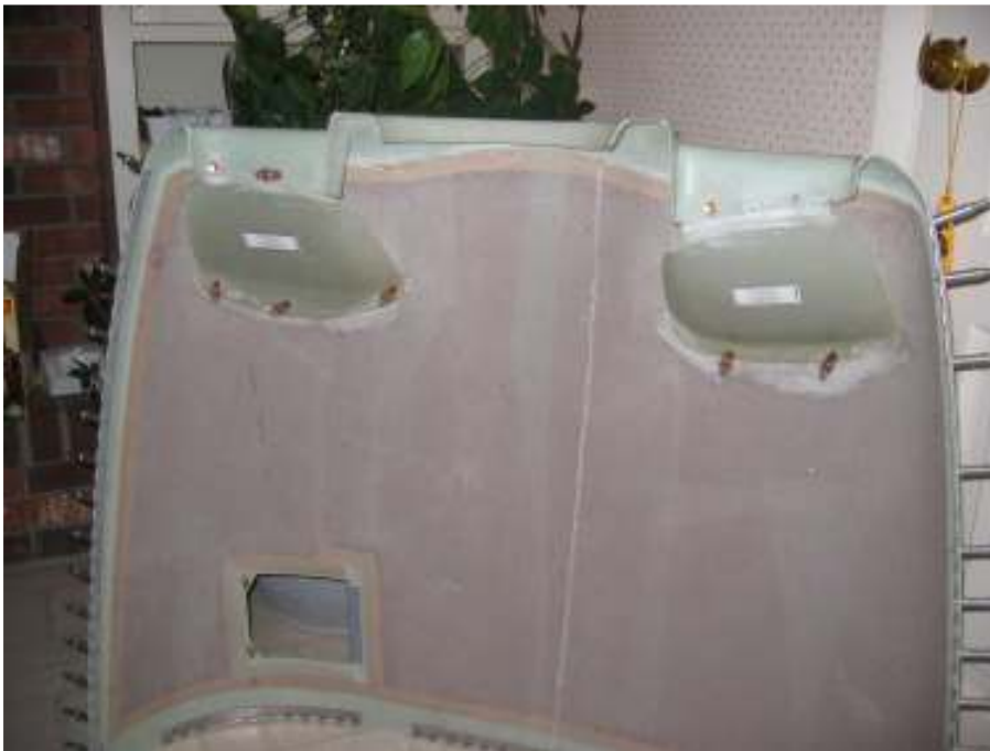
Upper air inlet glassed in Total time: 7 hours (913 hrs)
