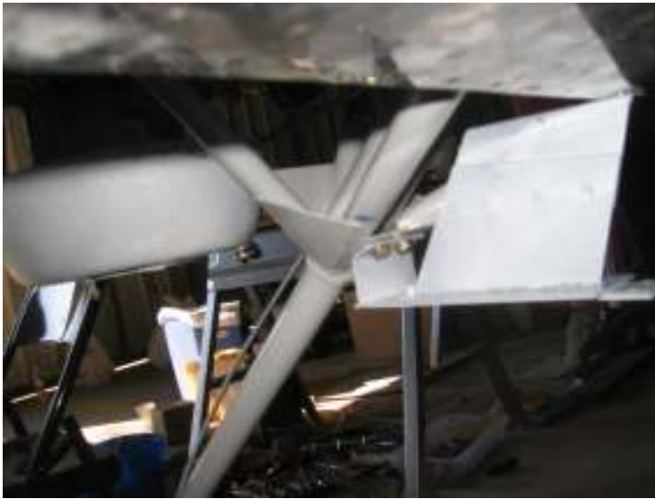
Bolt on main gear leg cover bracket (both bolts) One more layer of glass for air inlet fairing
