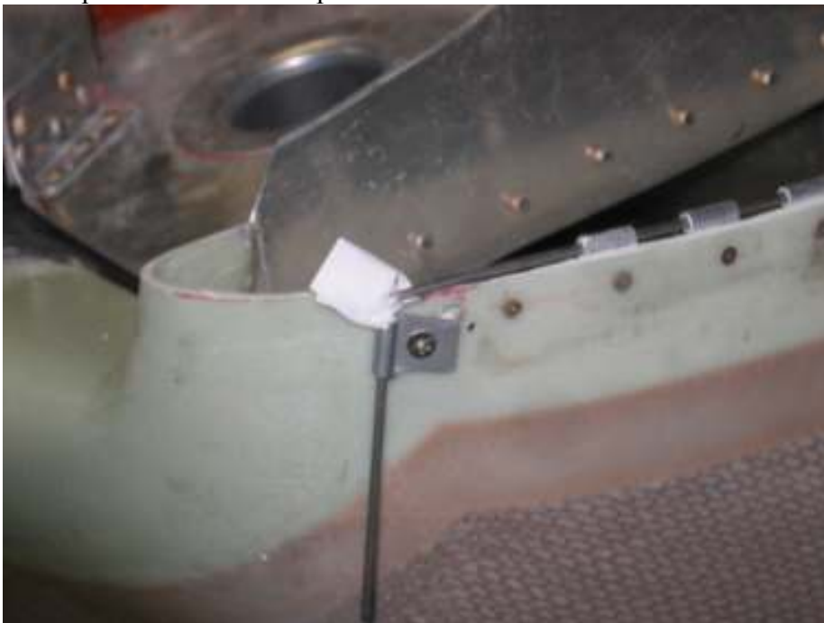
Install platenuts on lower cowl for hinge pins Total time: 5 hours (1000 hrs)
