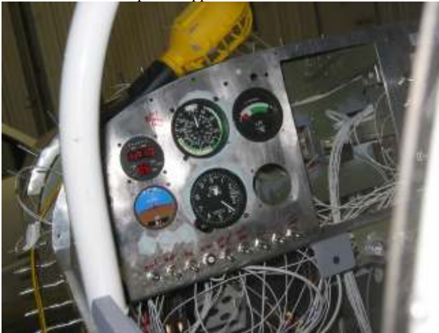
Wire clock and turn and bank Partially sealed baffle using high temp RTV Total time: 8 hours (980 hrs)
