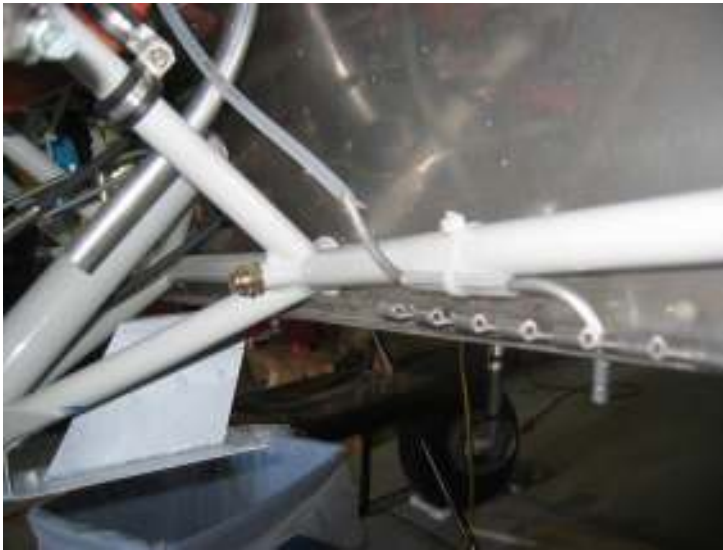
Install fuel overflow tube
