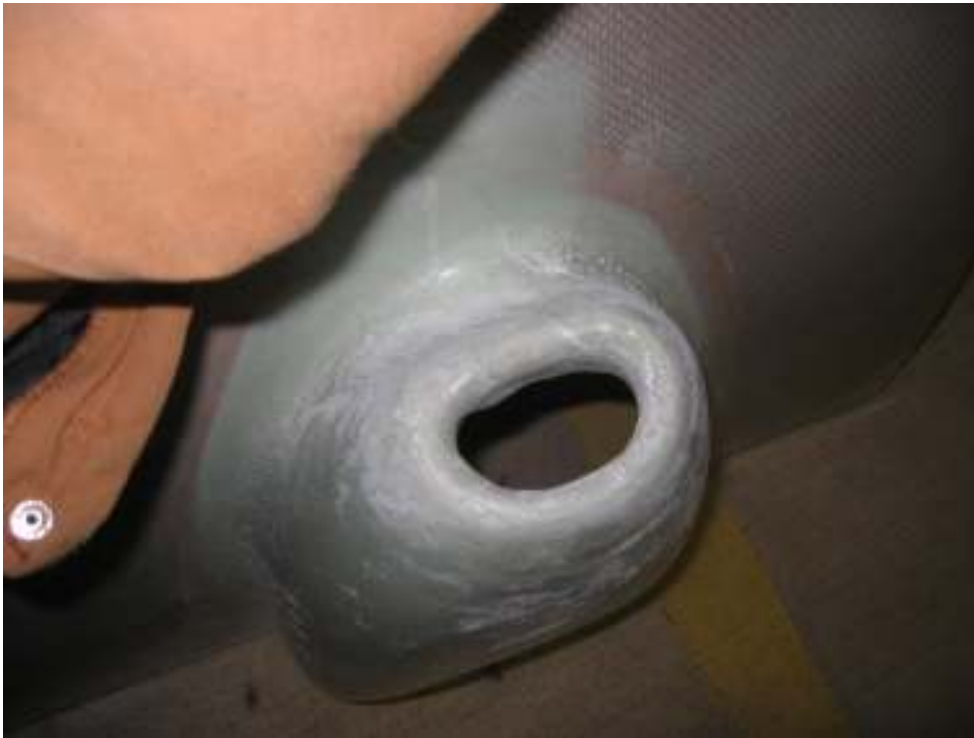
Sand cowl inlet Red RTV filling baffle gaps Total time: 4 hours (995 hrs)
