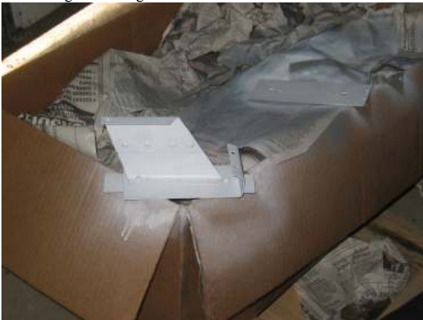
Prime and paint bottom cowl nose gear gap bracket Install air seal for air box
