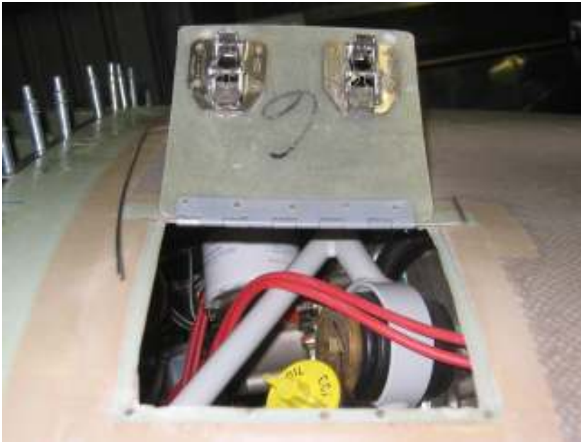
Install oil door latches Modify oil door opening on upper cowl and glass in strike plate
