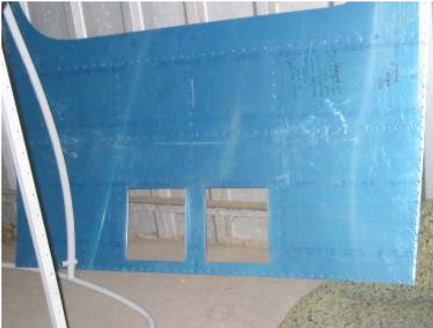
Cut upper skin access holes
