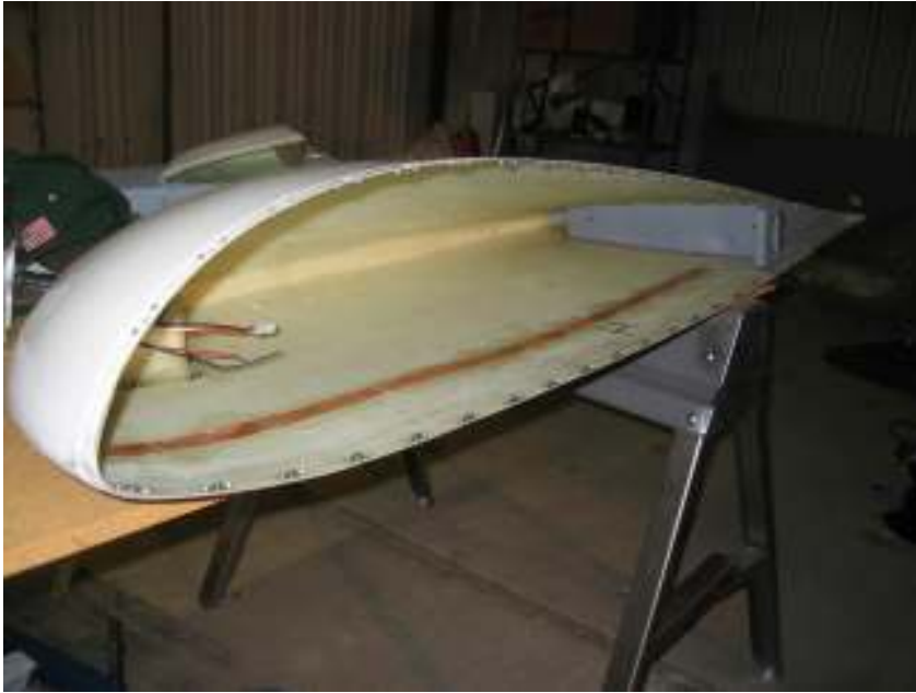
Glass in marker beacon antenna in right wing tip
