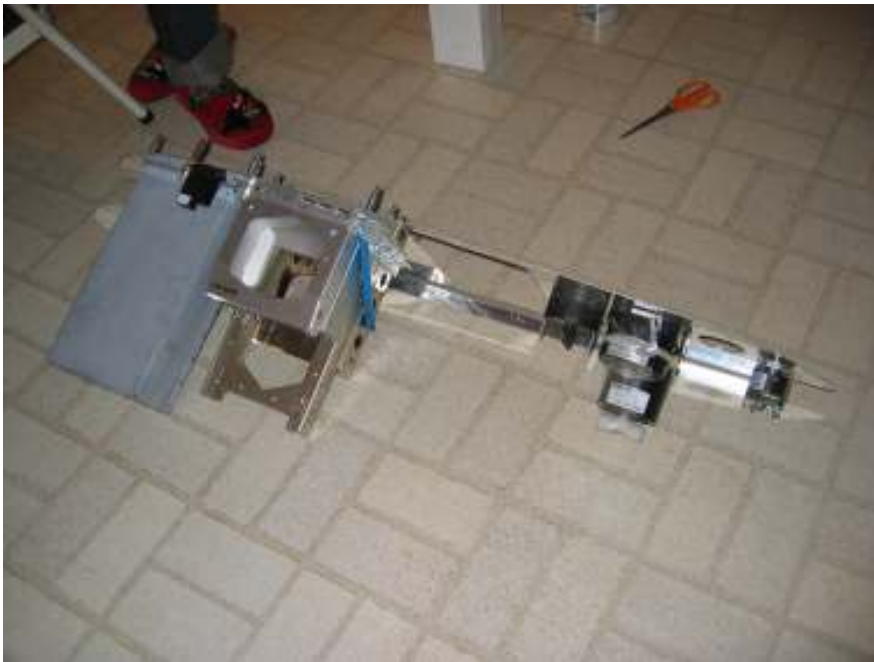
12/23/2005, Friday Cut opening for radio rack on subpanel
