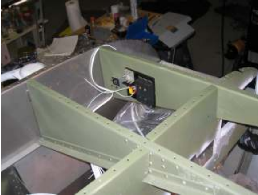
Mount E-bus and diod for E-bus
