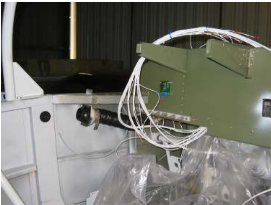
Enlarge eyeball light holes, drill mounting holes, wire eyeball lights Mount dimmer circuit board Misc. wiring Total time: 7 hours (635 hrs)
