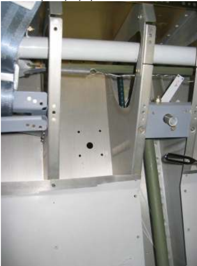
Drill mounting holes for belly bend COM antenna
