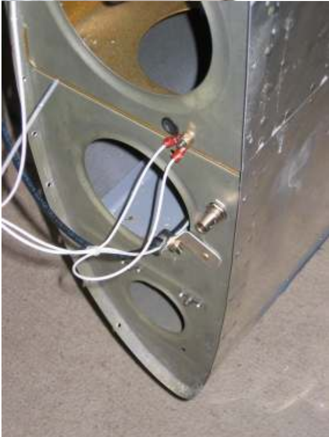
Wing wiring – nav, landing/taxi light Wire for pitot
