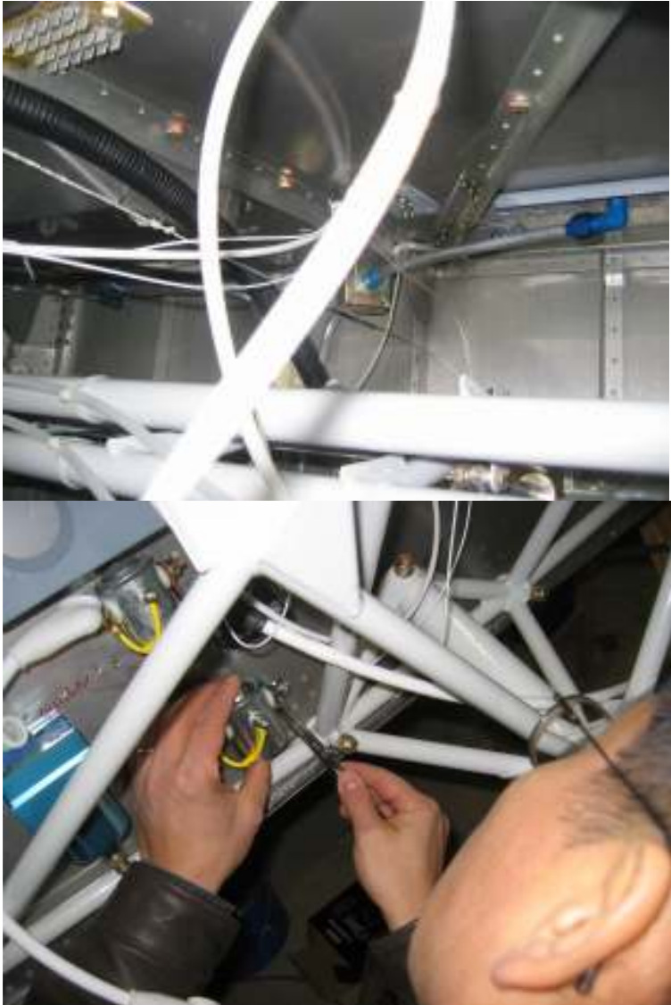
Rivet last rivet on left rear canopy skirt
