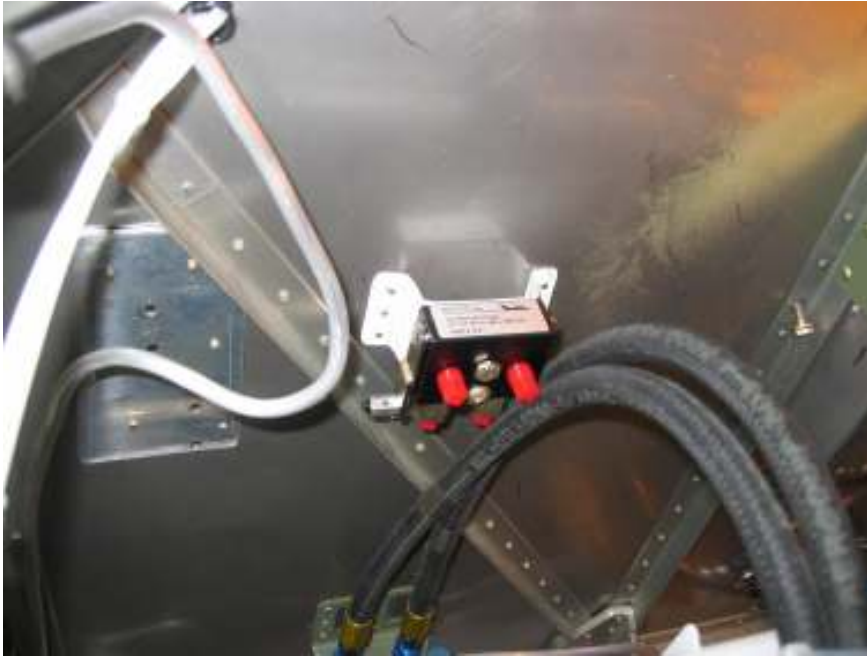
Rivet parking brake mount
