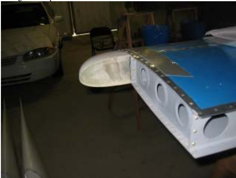
HS left side tip riveted in
