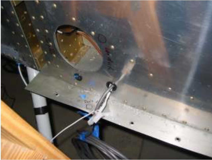
Drill through side fuselage for wire entry
