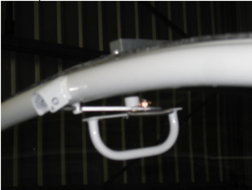
Finish canopy latch Total time: 6 hours (577 hrs)
