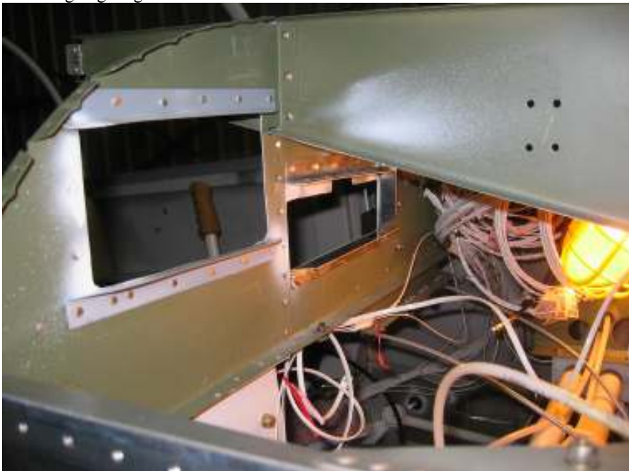
Rivet angles for the radio opening on subpanel
