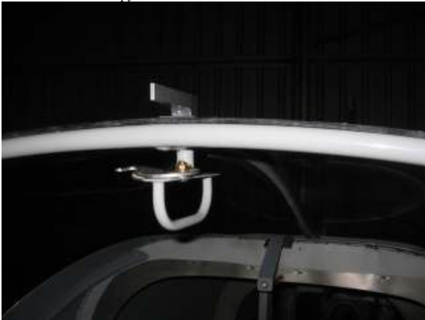
Grind down more on canopy latch tube Drill canopy latch handle to the tube (top), tap it.
