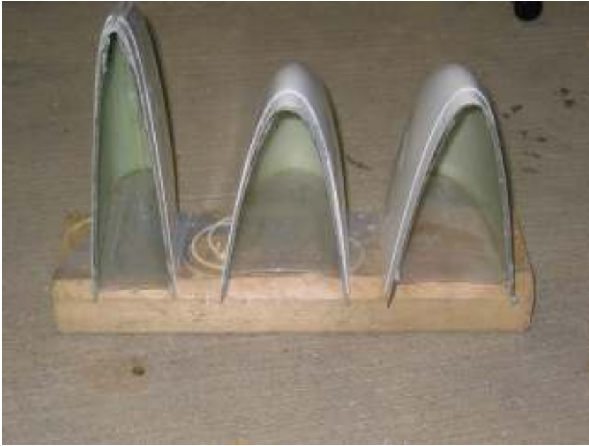
Remove cardboard support from tips, trim edges, glass in support from the back
