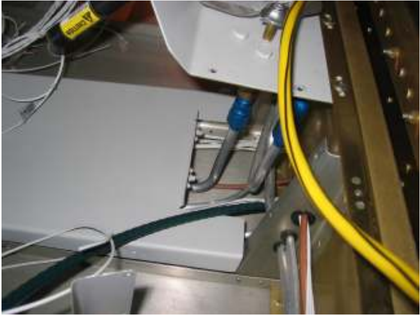
Finish fuel line on the floor
