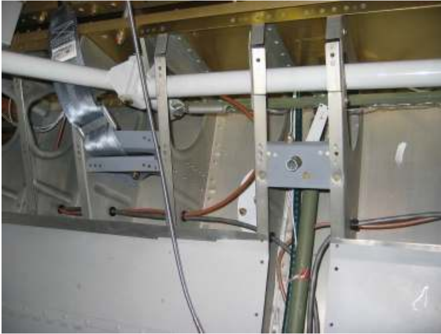
Re-route strobe wires
