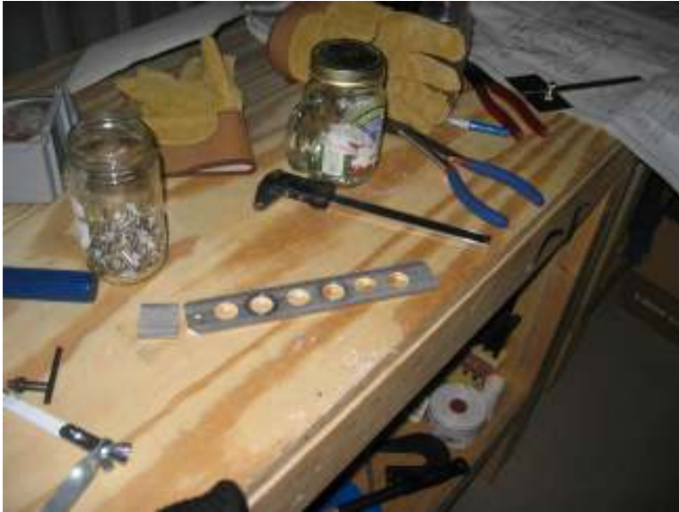
Drill auxiliary battery tray top brace
