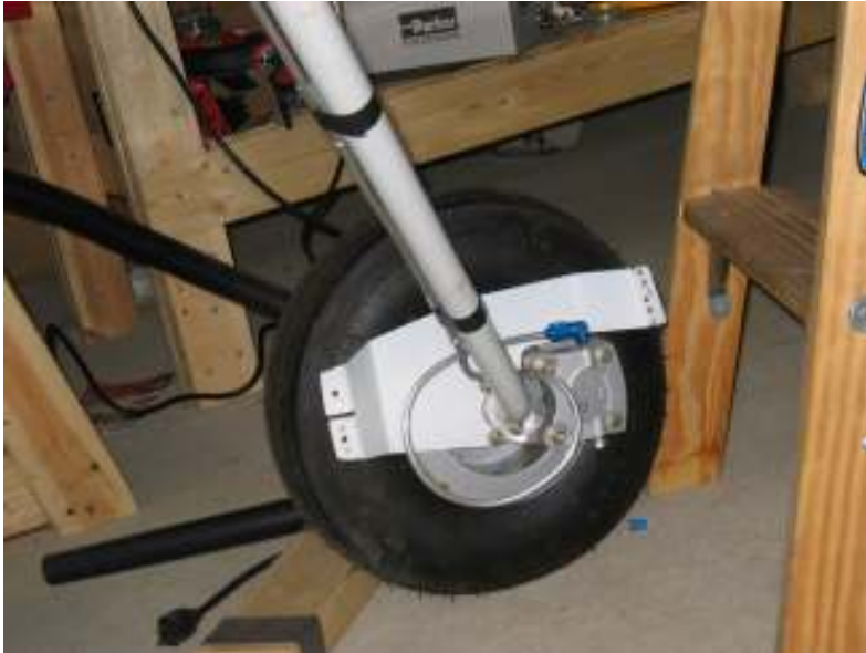
Install plastic tube to protect brake lines Total time: 3 hours (551 hrs)
