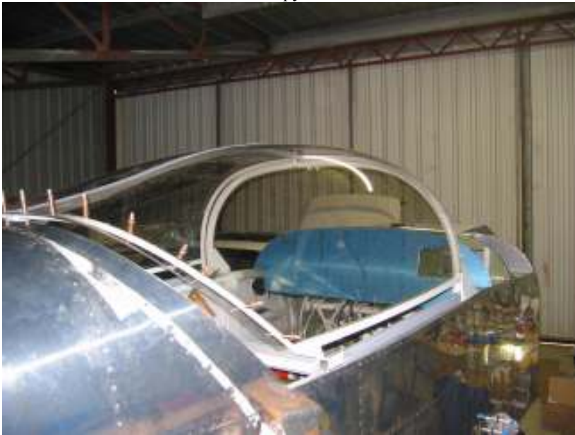
Enlarge holes in canopy and rivet front and top.
