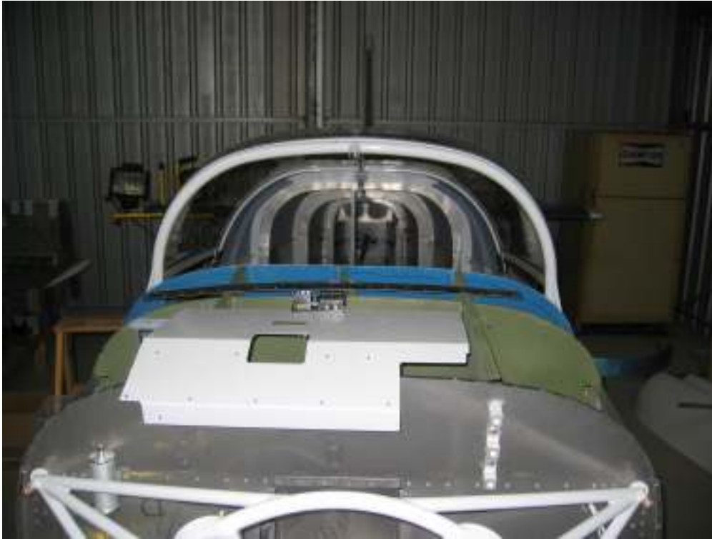
Remove all panels in rear cabin
