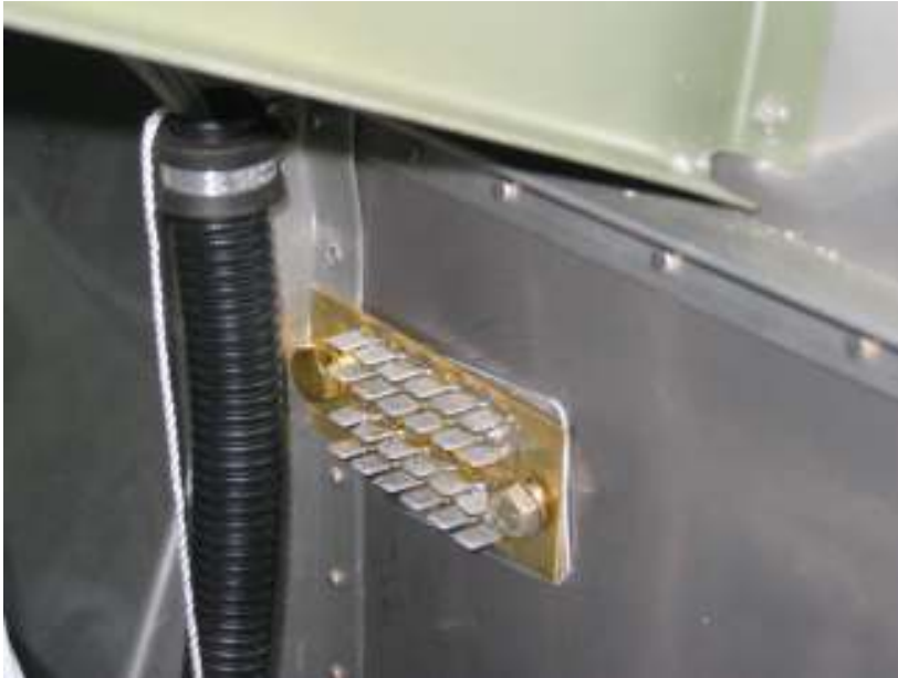
Cut shim for the firewall ground tab and drill the hole and mount it.
