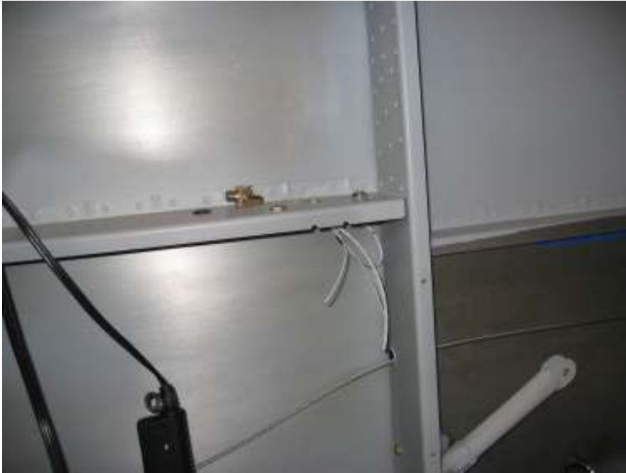
Re-route mike and phone cables, drill for snap on bushing, solder co-pilot phone jack Route co-pilot PTT wire back to the panel
