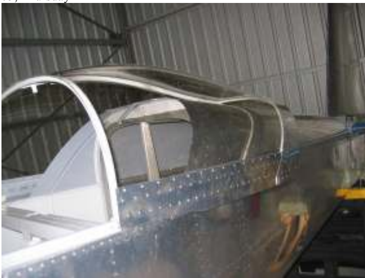
Finish riveting left side canopy skirts
