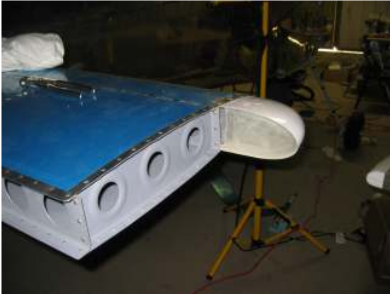
HS right side tip riveted in
