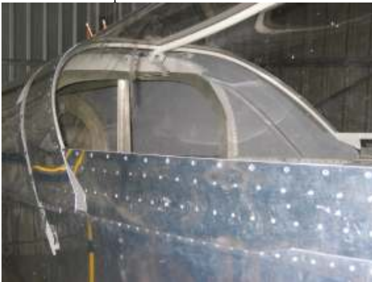
Rivet right side of the canopy skirts
