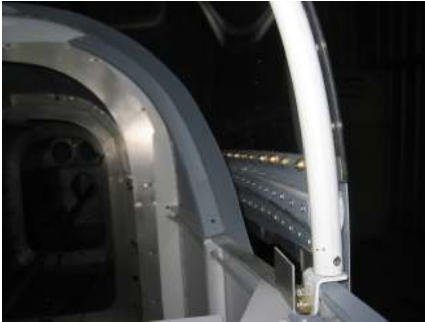
Fasten screws to canopy side
