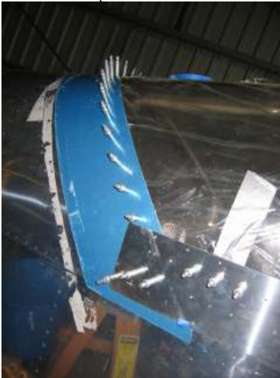
Drill right canopy rear skirt
