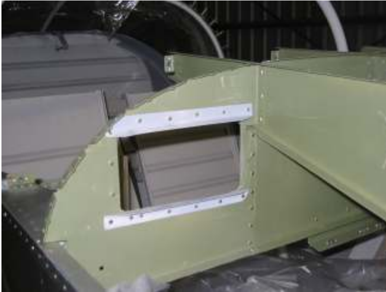
Cut hole in sub-panel and mount reinforcement angles
