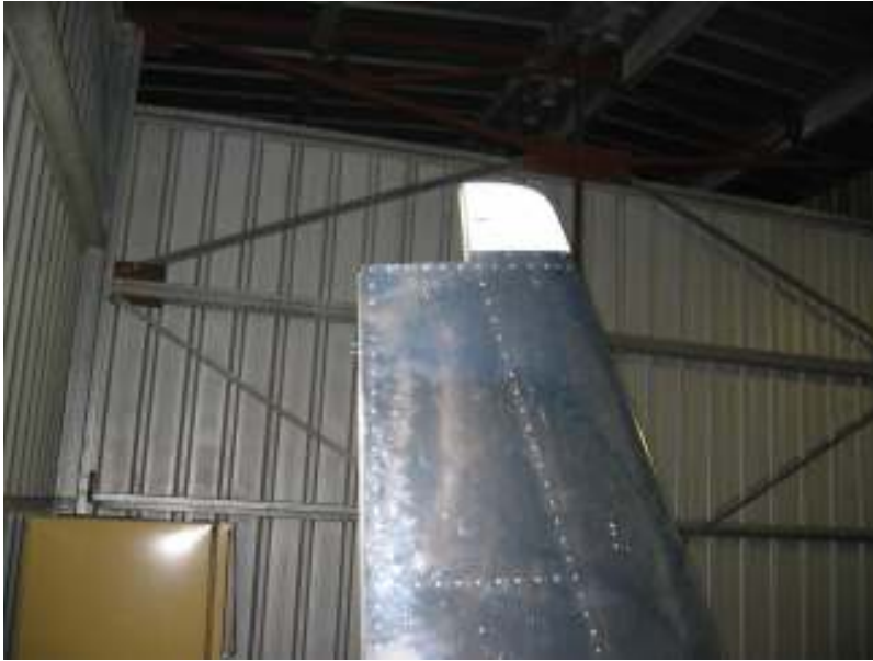
VS tip riveted in
