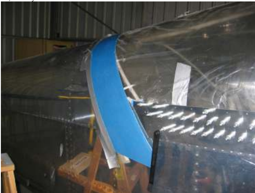
Bend canopy rear skirt Try to pump brake fluid again, failed. Total time: 3 hours (560 hrs)
