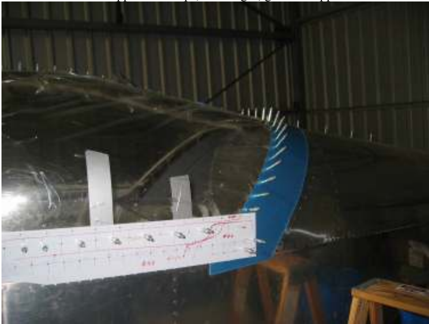
Drill the left side rear canopy skirt
