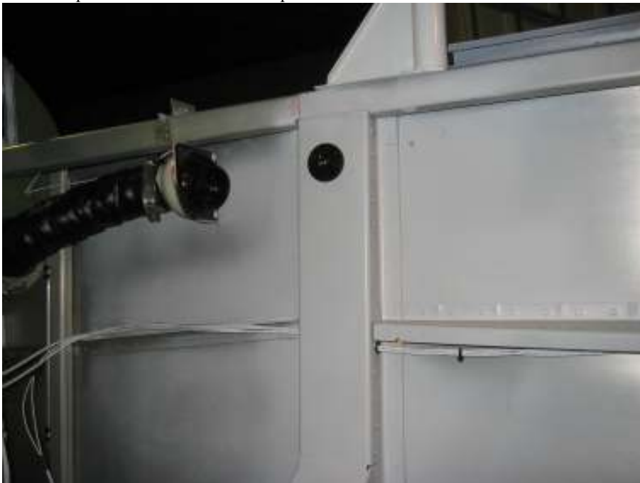
Re-route mike and phone cables, drill for snap on bushing, solder co-pilot phone jack Route co-pilot PTT wire back to the panel
