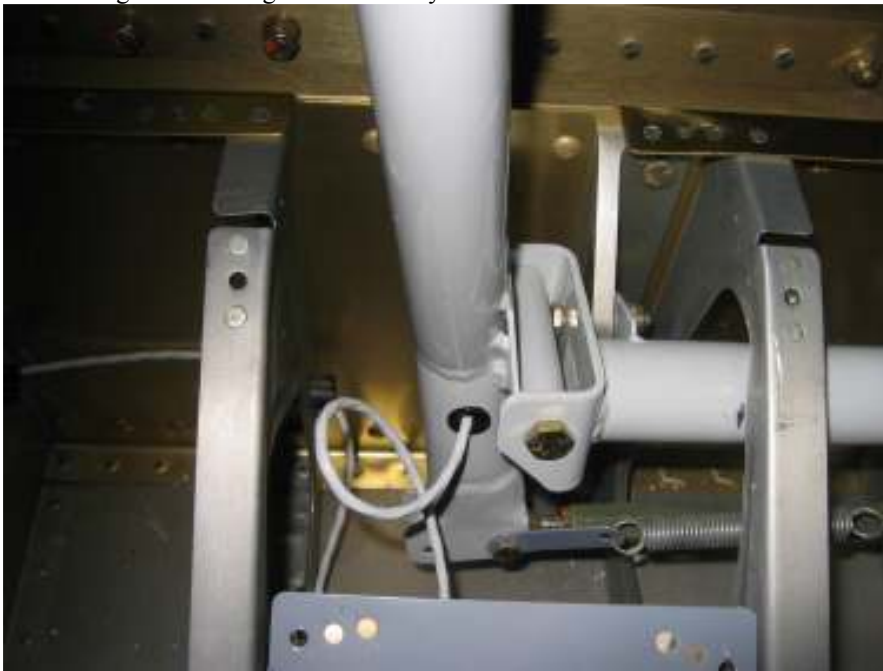
Drill hole on stick for PTT wire, fasten wire on fuselage
