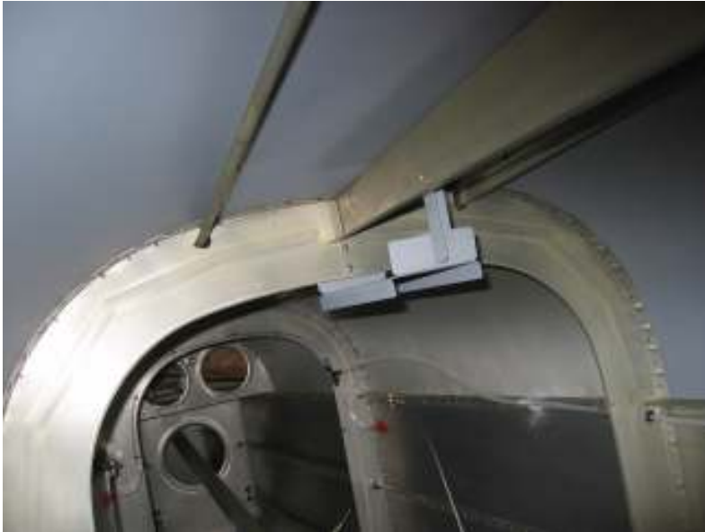
Build mounting bracket for GRT magnetometer Prime and mount the mount bracket Total time: 8 hours (452 hrs)
