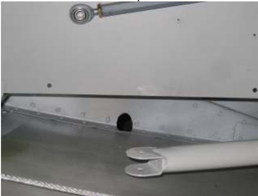
Drill holes for flap control rods Total time: 5 hours (373 hrs)
