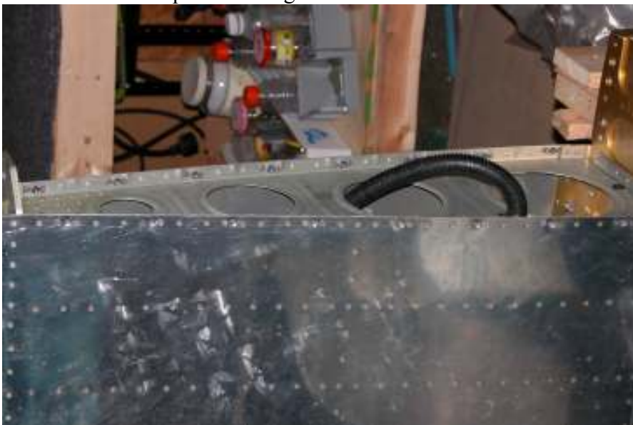
Replace and finish nutplates for right wing root
