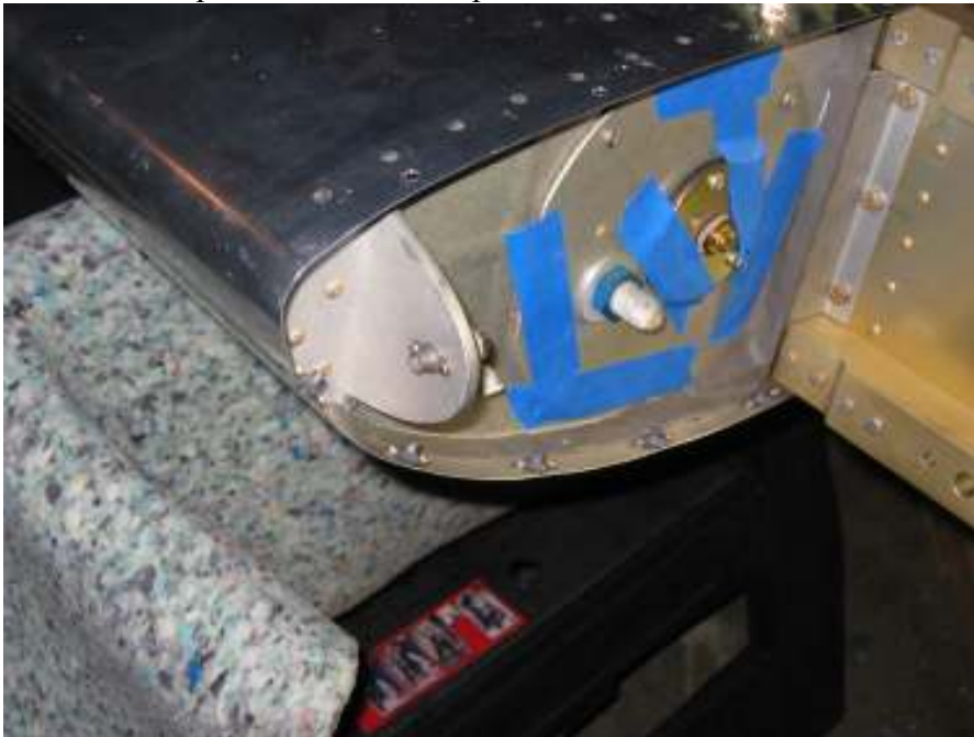
Rivet and torque elevator rear stop
