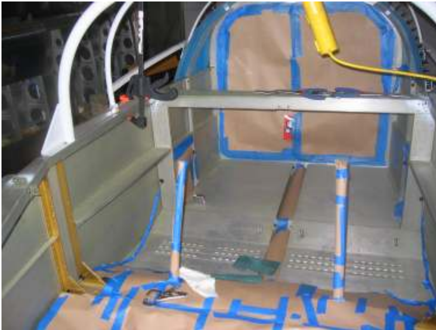
Drill for roll bar (time consuming, perpendicular angle is close)
