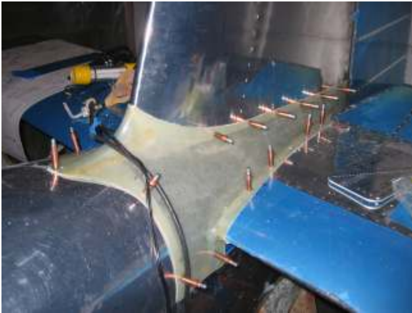
Trim empennage fairing, match drill holes for #6 screws, heat gun change shape Locate ELT antenna location at the tail
