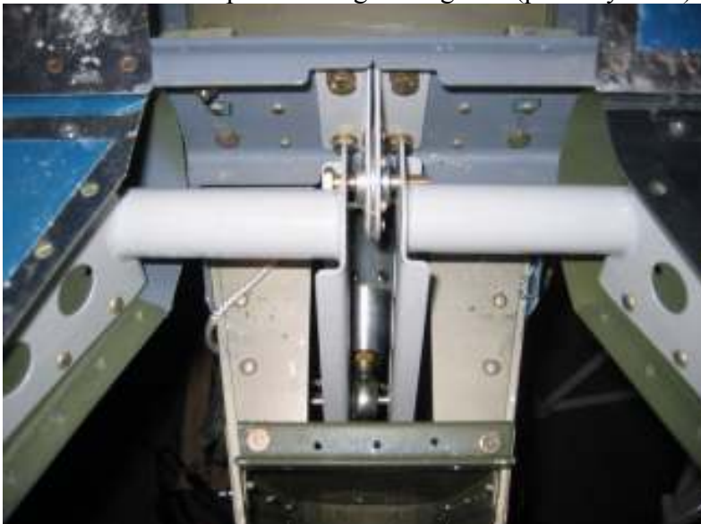
Install elevators to HS and drill holes on the horns
