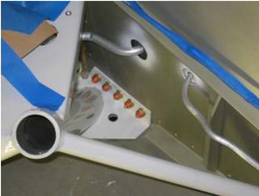
Enlarge brake line holes and torque gear mount bolts (only on the side wall)
