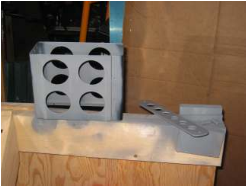
Finish most of the battery tray except two dimples
