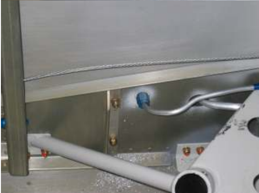
Drill fuel tank mount brace (still need to drill the 1/4" hole)
