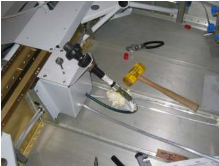
Install manual elevator trim cable
