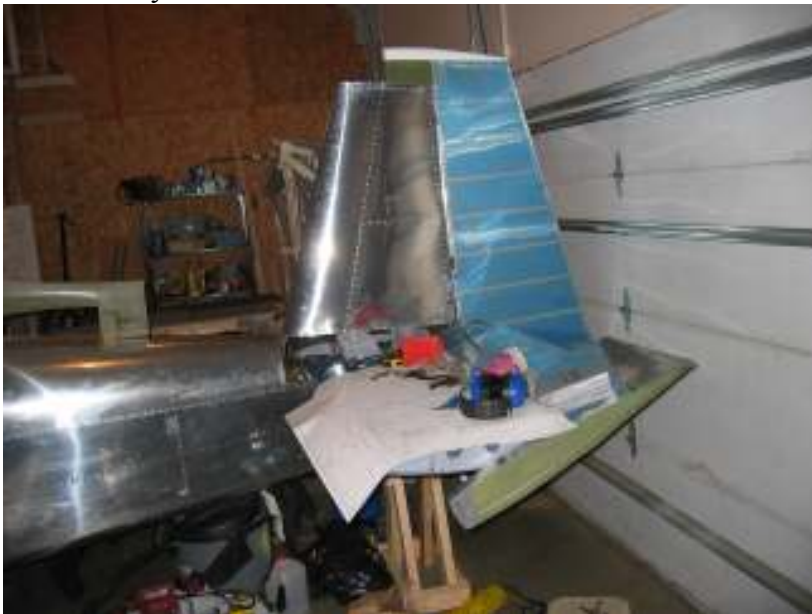
Test mounting left elevator Drill holes for VS rear spar Drill front mounting brace for VS Cut rubber channel for HS fairing
