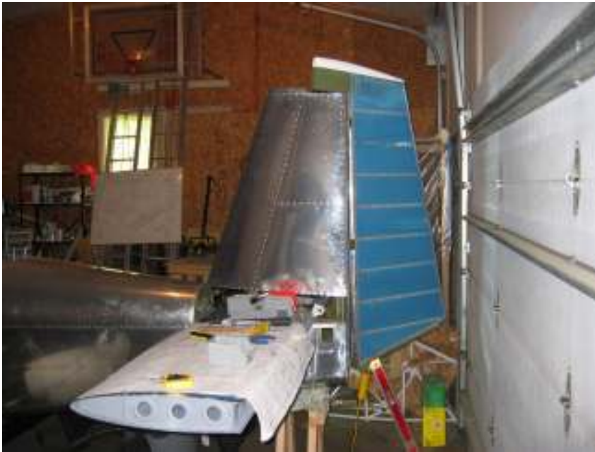
Double check the straightness of VS hinge braces (pass) Total time: 4 hours (348 hrs)
