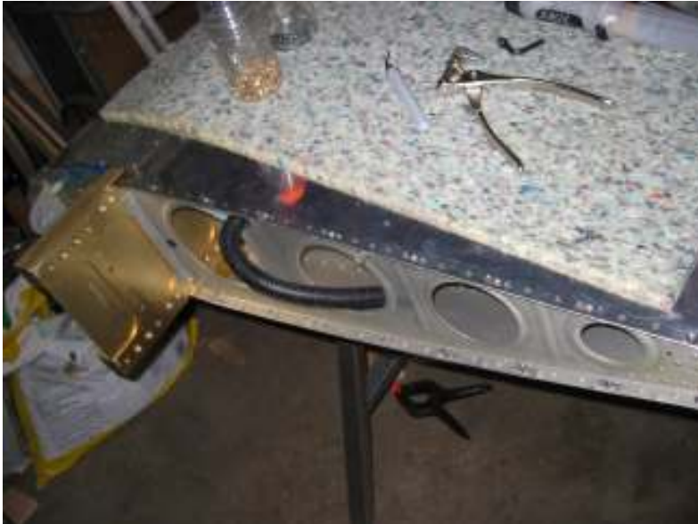
Drill and install nutplates on right wing root (partially done)
