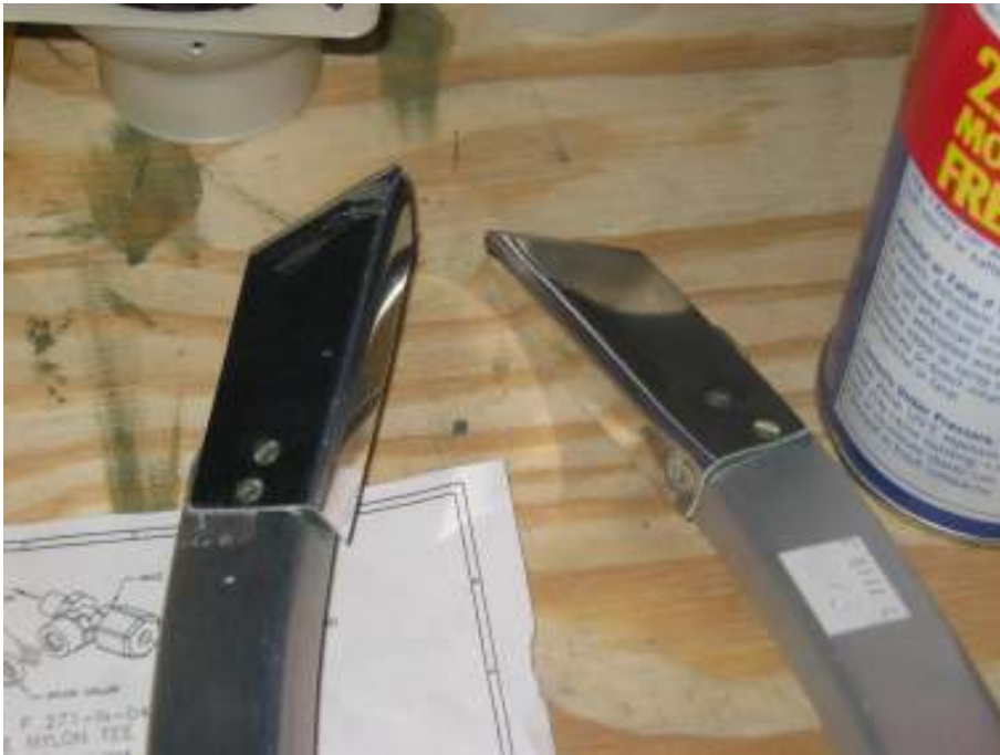
Rivet extension to F6111 Prime roll bar mounting spacer
