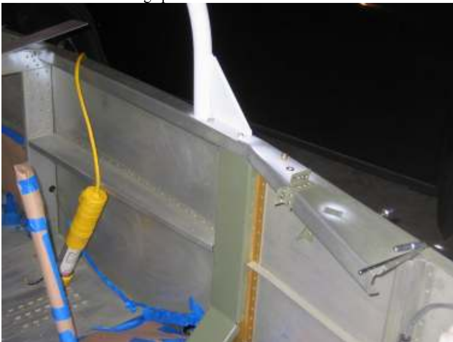
Mount front bolts for roll bar
