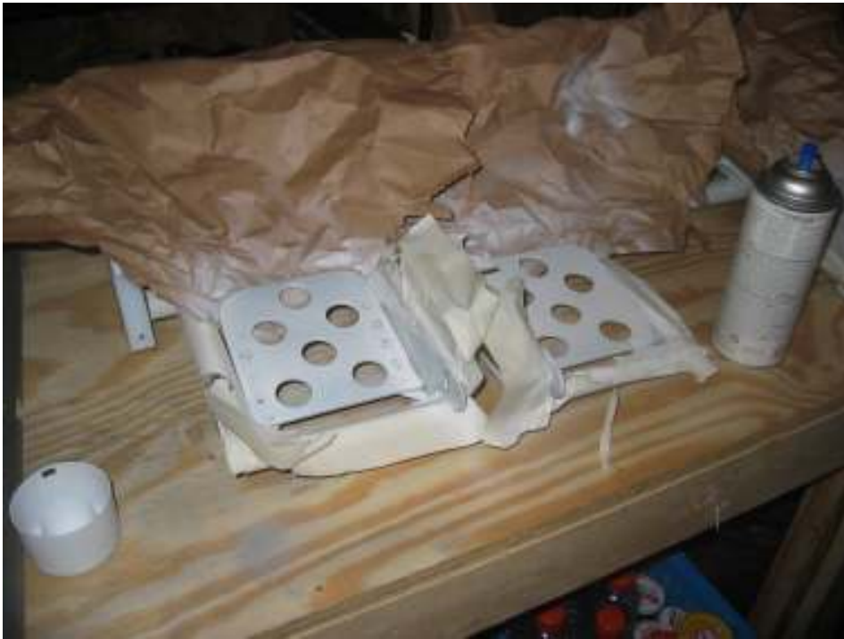
Prepare brake paddles for paint Total time: 4 hours (334 hrs)
