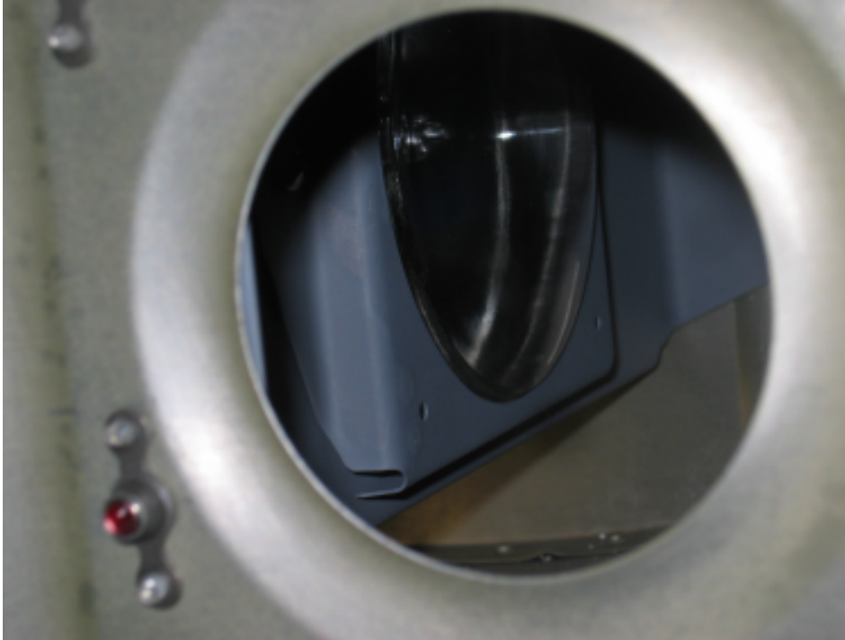
Finish both leading edge light lenses and light fixture
