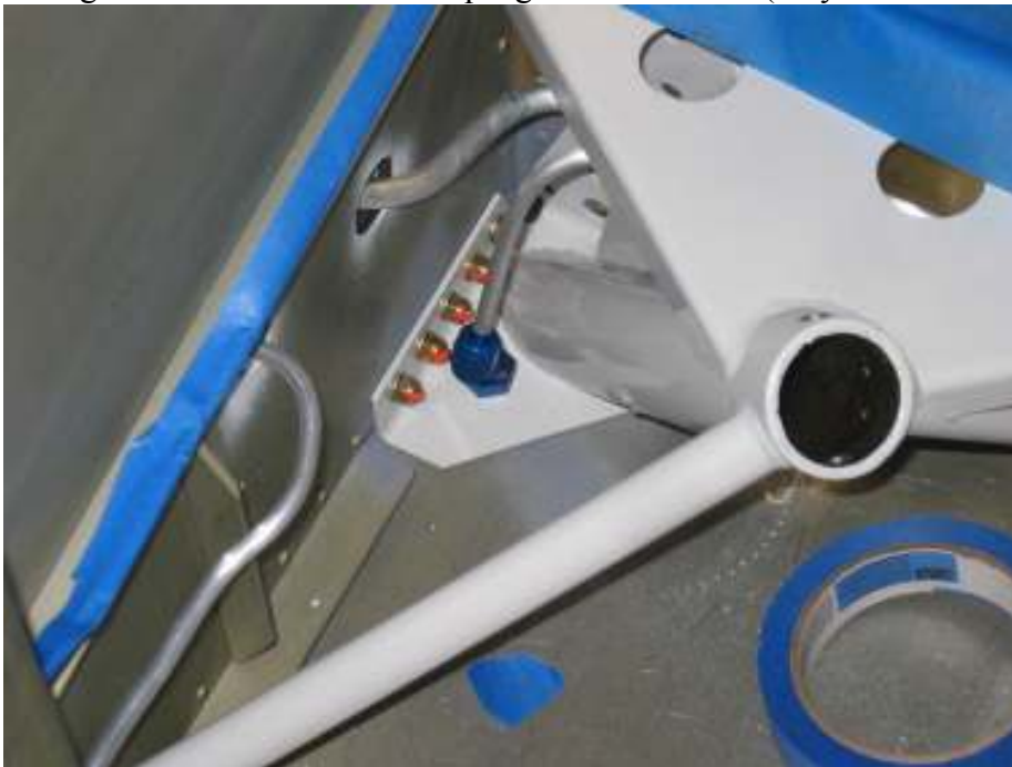
Partially installed brake line for the right side, There is a ding on the right side fuel line. Need to replace it.
