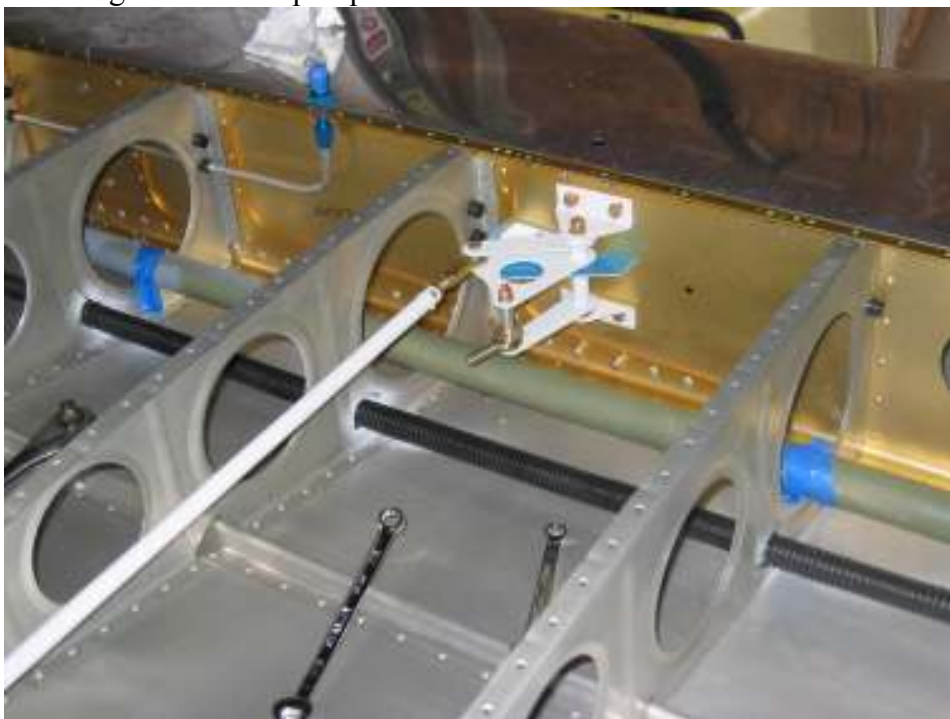
Set both aileron positions, finalize wing control ballcranks
