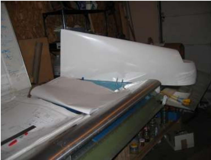
Mark wing tip for cutting
