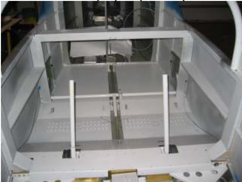
Finish most of the battery tray except two dimples
