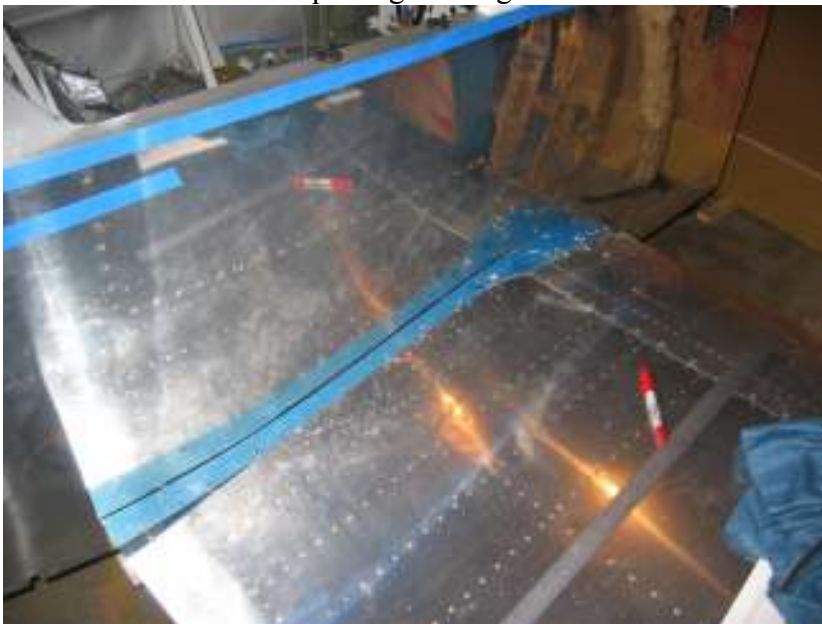
Match drill wing root fairings (drill nutplate holes on wings)
