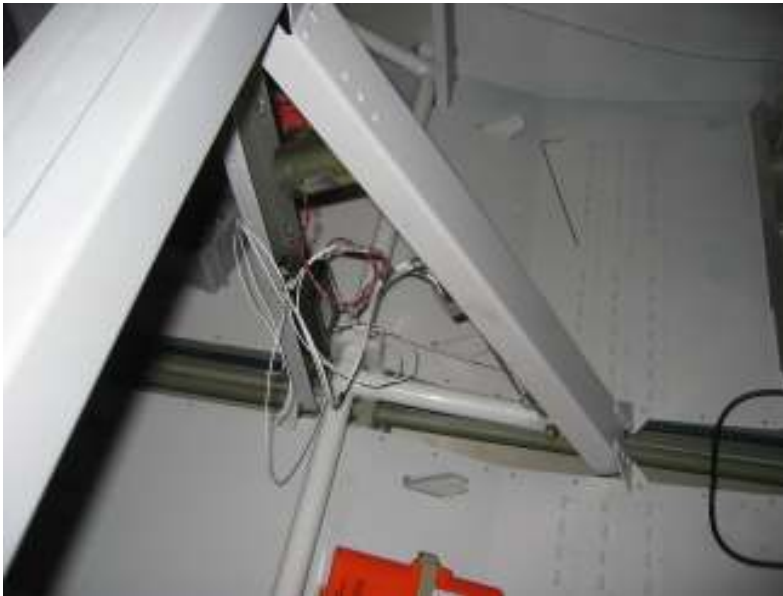
Mount rudder control column with actuator and control module
