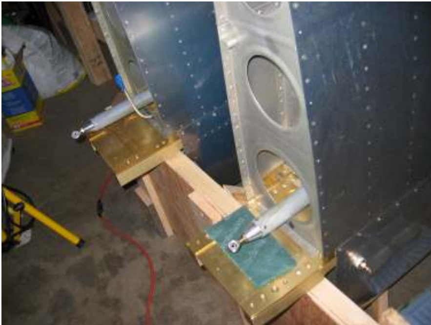
Finished aileron and elevator pushrod end riveting
