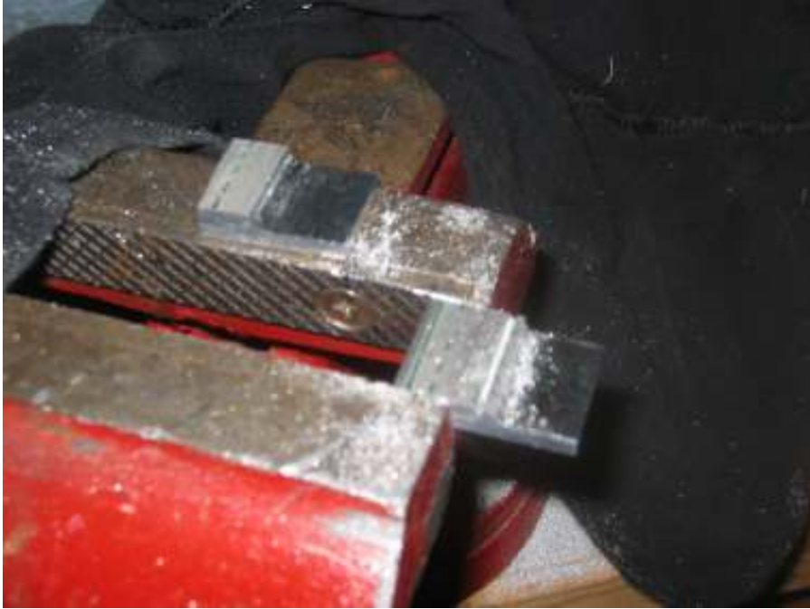
Fabricate brackets for roll bar attachment
