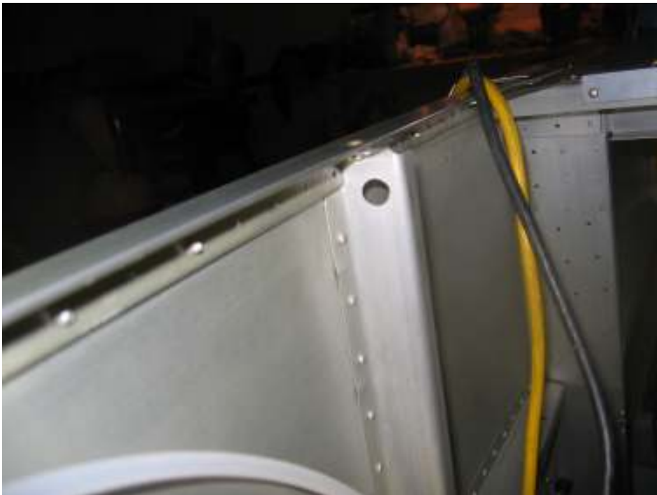
Drill hole for static line
