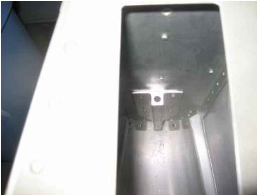
Drill hole for tail tiedown
