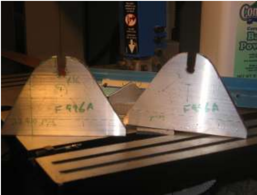
Fabricate F996A wing tank mounting braces, still need to bend them and smooth edges
