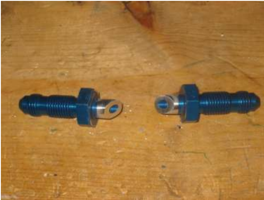
Grind 45 degree angle for vents
