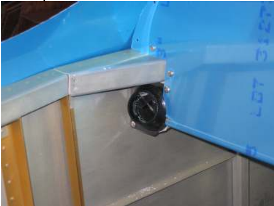
Drill fresh air outlet mounting brace Nutplate under the right
