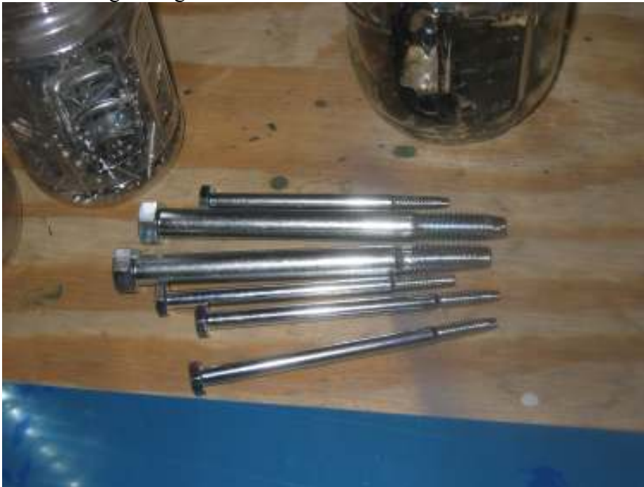
Grind hardware bolts for wing mating Total time: 7 hours (292 hrs)
