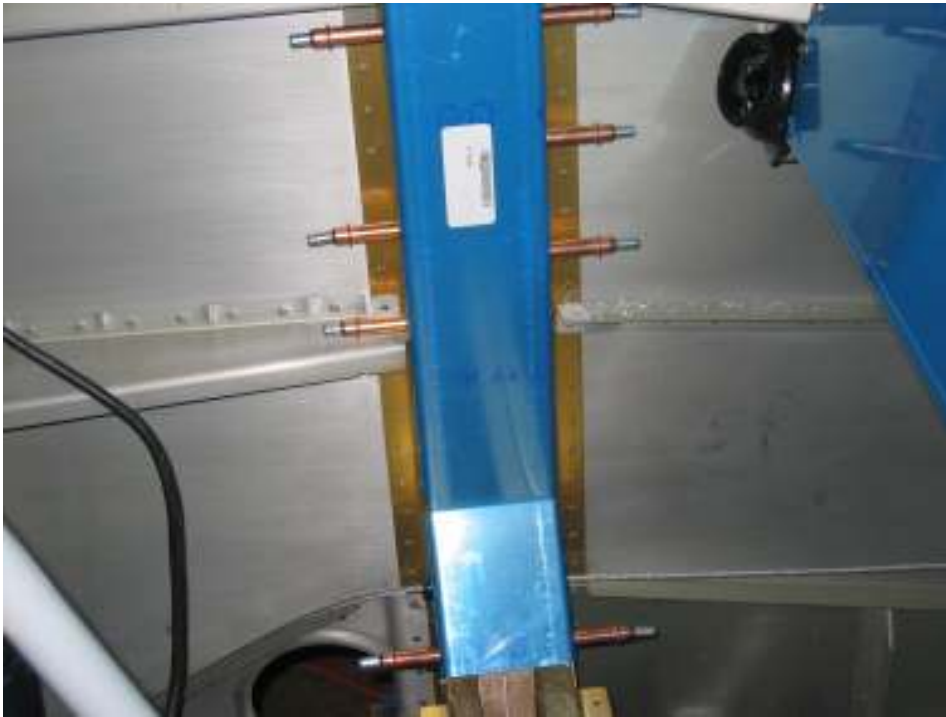
Match drill center column cover (left) Total time: 5 hours (238 hrs)
