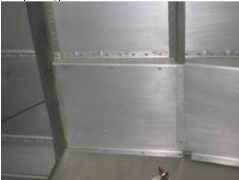
Close off baggage compartment rear side panels
