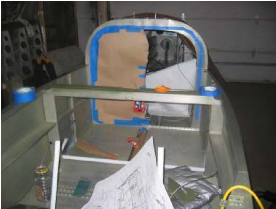
Begin prepare to mask for interior painting Total time: 2 hours (277 hrs)
