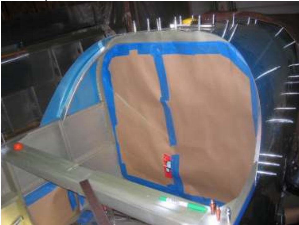
Fit curved support Flare and install left vet tube, cut one of the screws short to avoid hitting the skin
