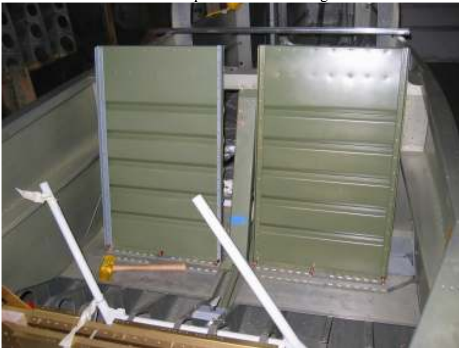
Finish the 2 nd seat back Total time: 4 hours (208 hrs)
