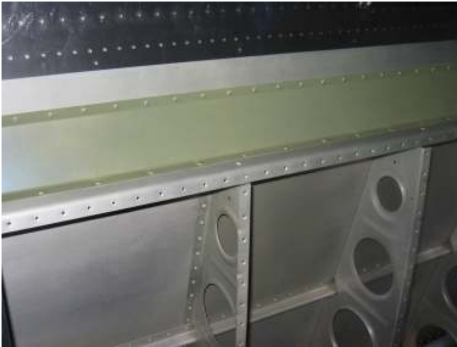
Fix bad rivets on right wing flap fairing Countersunk already lightly dimpled holes on the rear wing spar
