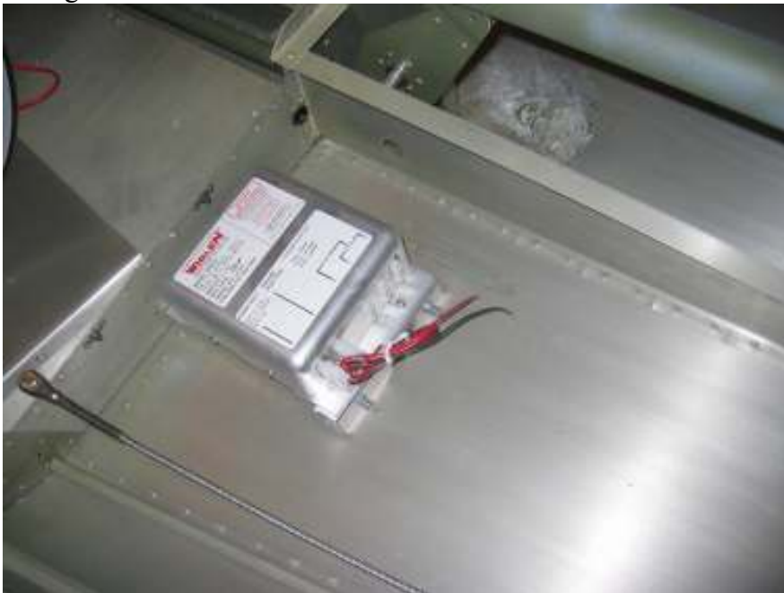
Fabricate brace for flasher power supply mounting behind the baggage compartment
