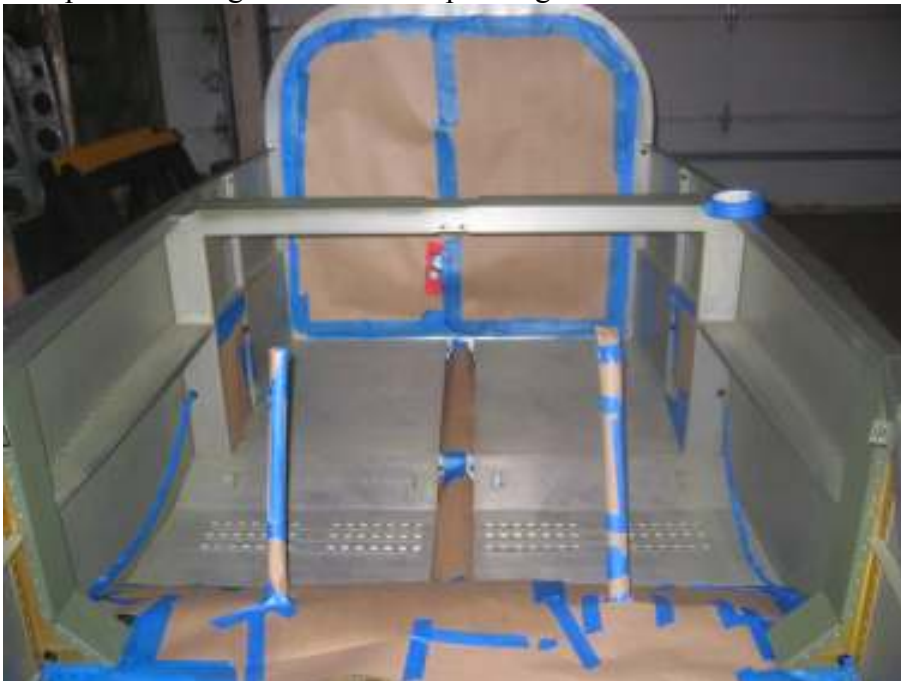
Remove flap control column
