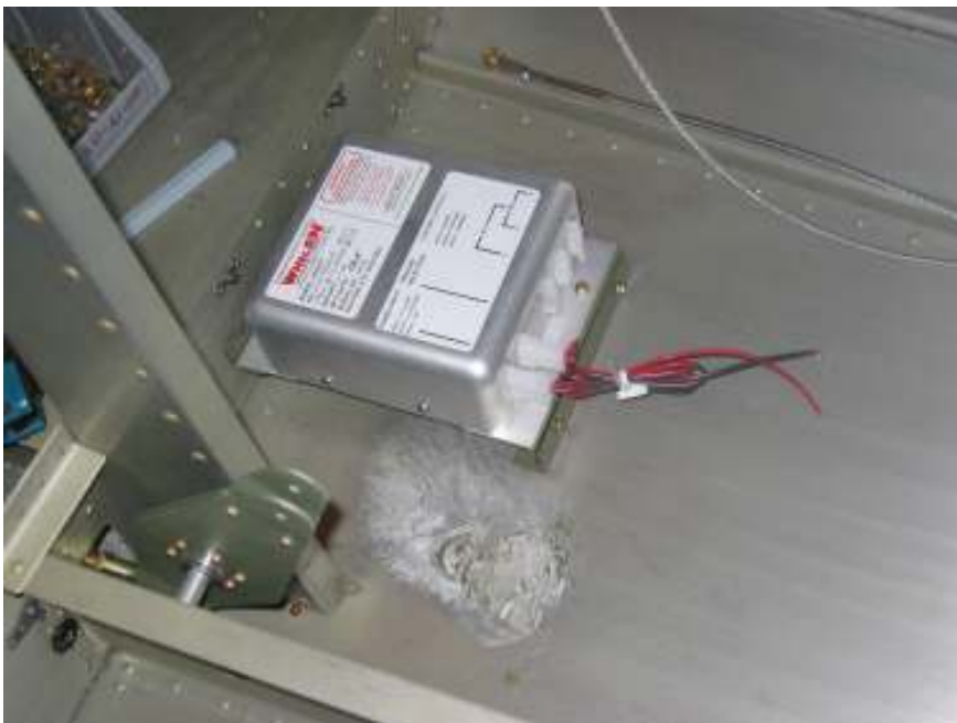
Install flasher power supply behind the baggage compartment
