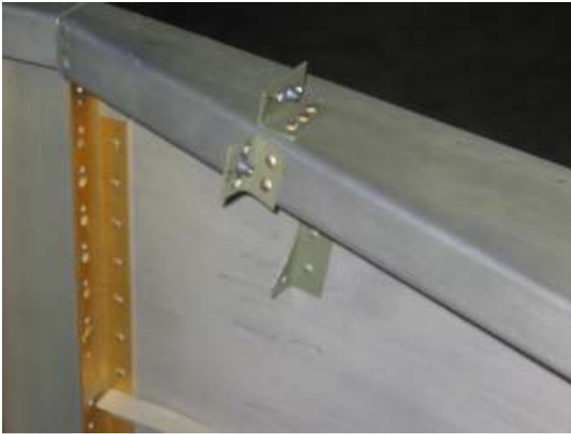
Rivet panel support and air outlet braces
