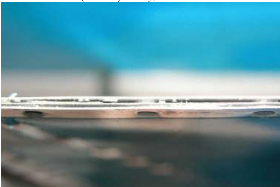
Rudder trailing edge after riveting
